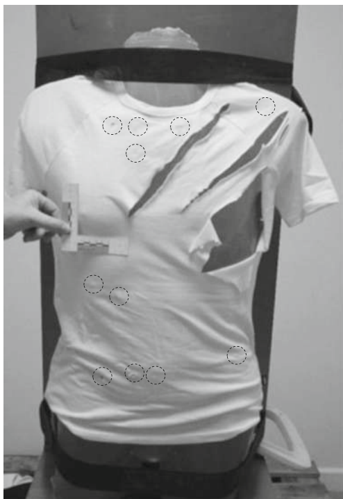
Fig. 4 Post-attack analysis of an attack by an expert user on a PermaGel™ torso wearing a white 100% cotton T-shirt (small impacts made with weapon tip are circled). Cowper, E., Mahoney, P.F., Godhania, K., Carr, D.J. and Harrison, K., A pilot study examining garment severance damage caused by a trained sharp-weapon user, Textile Research Journal , 87, 1287–1296. Copyright © 2017 (Sage Publications). Reprinted by permission of SAGE Publications
