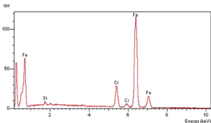
Fig. 1. Case 6 – SEM picture of many irregular-shaped metallic fragments (bright areas) of iron and chromium, as shown in the spectrum on the right.
