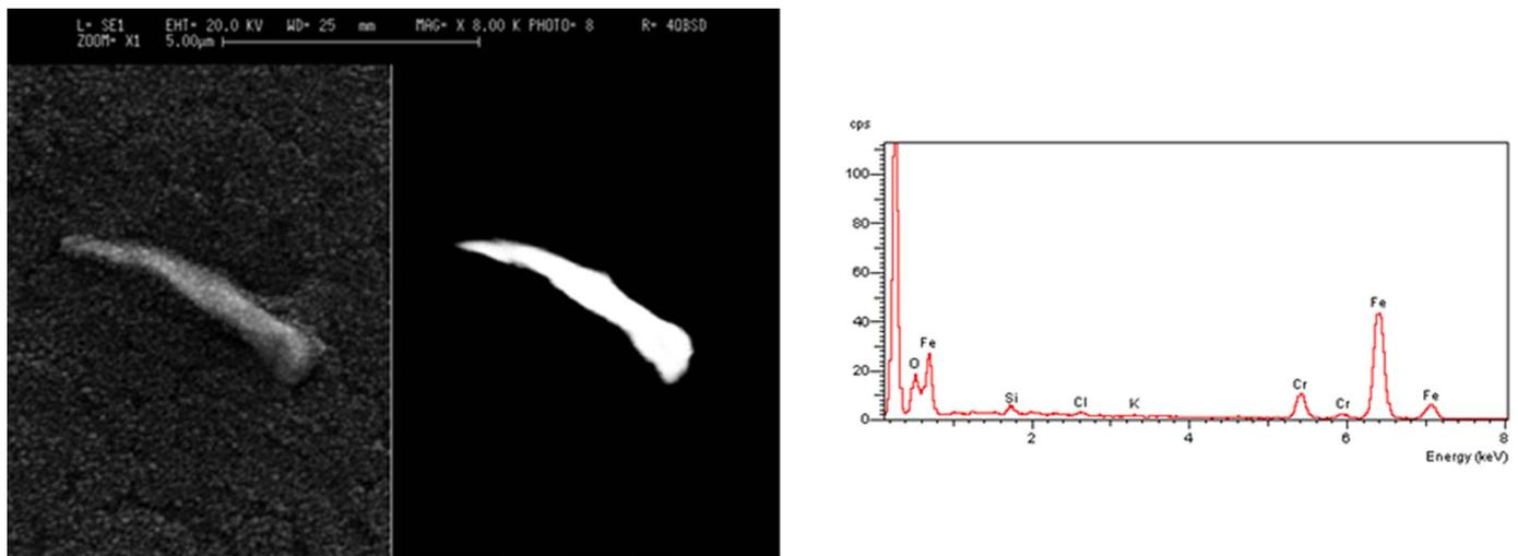
Fig. 2. Case 10 - SEM picture of metallic fragment with a “comma”-shape ( $5,5 \mu \times 0,7 \mu$ ) of iron and chromium, as shown in the spectrum on the right.
