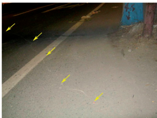
Figure 2. Scratches formed by friction between the motorcycle and the ground showed the trajectory of motion of the motorcycle after the collision with the pillar (intraday).
