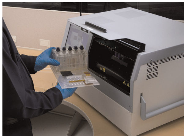
Figure 3 A technician is loading the 5 sample Biochip into the Rapid DNA instrument.
